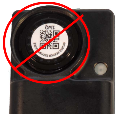
Filter cartridge is installed upside down in UPAS
